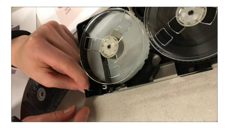
One of the tricks we learned while in DC at Bootcamp was audio cassette and VHS tape rehousing. This is for when a patron comes in with a damaged tape and it needs to be put into a new case so it can be digitized without messing up our equipment or damaging the physical tape inside the housing.
